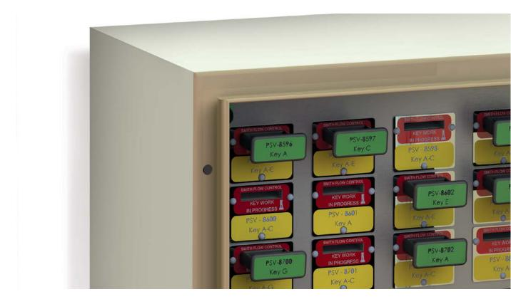
Simply by looking at the keys in your cabinet, you gain an overview of the status of your interlocked process systems. A cabinet with all its keys stored, indicates normal operation. Work is in progress when a key is missing from the cabinet.
