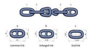
A swivelforerunner normally consists of: endlink - swivel - enlarged link - common link (as from 30mm chaincables)
