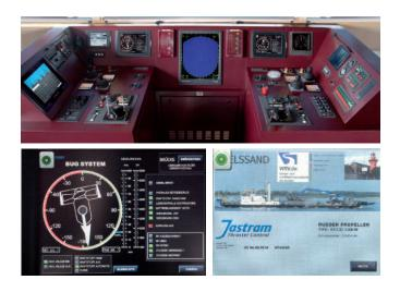
The UniProp can be controlled both from the bridge as well as on site. The equipment and the layout of the bridge can be easily altered to the customer's desire. This is achieved with a combination of lever units, buttons and analogue displays or touch panel technology.
