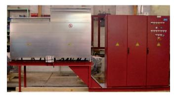
The rack-mounted 3-step drive with switch cabinet and resistor unit reduces onboard installation time.
