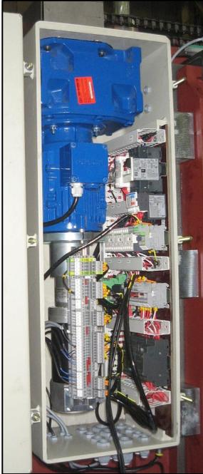
The CONDOR is a compact door which means that complete the drive unit, consisting of a geared motor for normal supply, a 24VDC motor (for emergency drive above bulkhead), electrical control plate and control levers are pre-mounted on the bulkhead plate which is welded to the door frame. The Rail extensions with support and bolts, two local hand generators for emergency drive, wheelhouse panel and emergency station are loose supplied.
