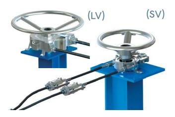
Operator stations are available in a variety of different gear ratios, providing a wide range of torque capabilities. A helically wound steel cable has a pitch the same as that of the cable gear. The precision gearcable interface provides a positive force to the helix cable, which travels through the flexible conduit to the valve station actuator.
